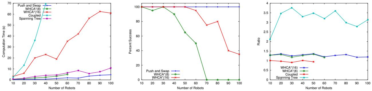
Fig. 10. Random grid experiment. All values are averages of 20 runs. (left) Computation time for varying numbers of robots using different techniques. (middle) Success rate for WHCA\*. (right) The ratio of solution lengths for various techniques against those computed by PUSH\_AND\_SWAP.
