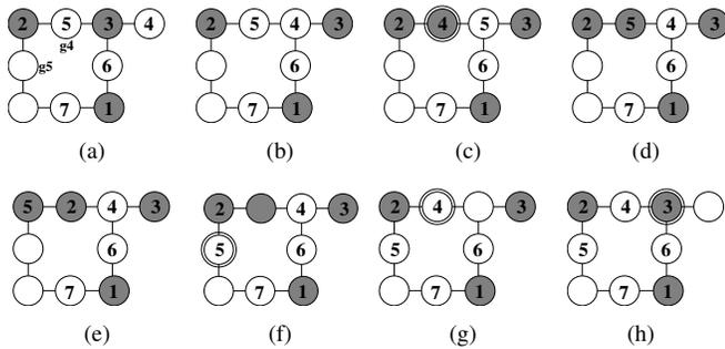
Fig. 5. RESOLVE: Vertices in  $\mathcal{U}'$  are shaded. (a) After robots 1, 2 and 3 have planned. (b) Robot 4 swaps with 3. (c) Resolve is invoked (3 was at goal). 4 swaps with 5 and reaches its goal. (d) Resolve called for 3 and 5; 5 swaps with 4. (e) 5 swaps with 2 invoking Resolve again. (f) 5 pushes to its goal; third Resolve is successful. (g) 4's goal is freed; second Resolve is successful. (h) 3's goal is free; first Resolve is complete.
