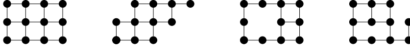
Figure 1.1: From left to right: a rectangular grid graph, a solid grid graph, a grid graph that is neither rectangular nor solid, a subgrid graph that is not a grid graph.
