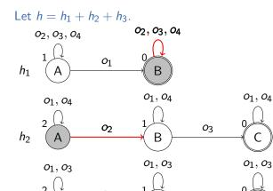
$\langle o_2, o_3, o_4 \rangle$  is a plan for  $s = \langle B, A, A \rangle$  but h(s) = 4. Heuristics  $h_2$  and  $h_3$  both account for the single application of  $o_2$ .
