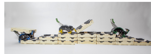
Harvard TERMES robots, based on termites
