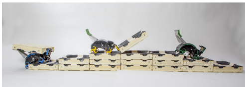
Harvard TERMES robots, based on termites
