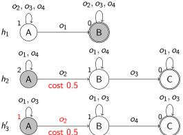
$\langle o_2, o_3, o_4 \rangle$  is an optimal plan for  $s = \langle B, A, A \rangle$  and h'(s) = 0 + 1.5 + 1.5 = 3 an admissible estimate.
