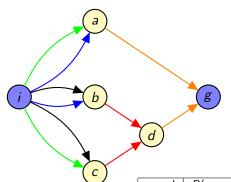
$$\begin{array}{l} o_{\text{blue}} = \langle \{i\}, \{a,b\}, \{\}, 4 \rangle \\ o_{\text{green}} = \langle \{i\}, \{a,c\}, \{\}, 5 \rangle \\ o_{\text{black}} = \langle \{i\}, \{b,c\}, \{\}, 3 \rangle \\ o_{\text{red}} = \langle \{b,c\}, \{d\}, \{\}, 2 \rangle \\ o_{\text{orange}} = \langle \{a,d\}, \{g\}, \{\}, 0 \rangle \end{array}$$
