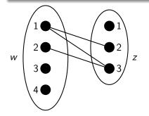
Arc consistency of w with respect to z and of z with respect to wis violated.
