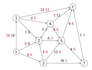
How hard is it to find a maximal flow? For example with the Edmonds-Karp algorithm in  $O(|E|^2|V|)$
