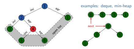
open list open organizes leaves of search tree with the methods: open.is\_empty() test if the open list is empty open.pop() remove and return the next node to expand open.insert(n) insert node n into the open list
