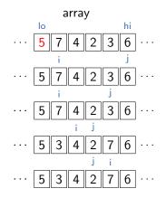
Pivot is at position lo. Initialize i = lo + 1, j = hi*i* to the right until element  $\geq$  pivot *j* to the left until element  $\leq$  pivot
