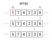
Pivot is at position lo. Initialize i = lo + 1, j = hi*i* to the right until element  $\geq$  pivot *j* to the left until element  $\leq$  pivot
