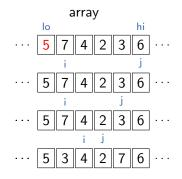
$\begin{array}{l} \mbox{Pivot is at position lo.}\\ \mbox{Initialize } i = \mbox{lo} + 1, j = \mbox{hi}\\ i \mbox{ to the right until element} \geq \mbox{pivot}\\ j \mbox{ to the left until element} \leq \mbox{pivot} \end{array}$
