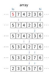
Pivot is at position lo. Initialize i = lo + 1, j = hi*i* to the right until element  $\geq$  pivot *j* to the left until element  $\leq$  pivot
