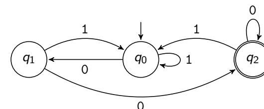
When reading the input 01100 the automaton visits the states  $q_0, q_1, q_0, q_0, q_1, q_2$ .
