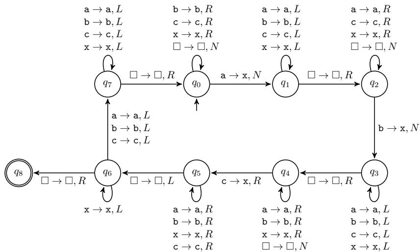
State  $q_0$  starts at the beginning of the input and reads the word from left to right until the first  $a$ . All symbols remain unchanged until the first  $a$  is replaced with an  $x$  at which time the TM
