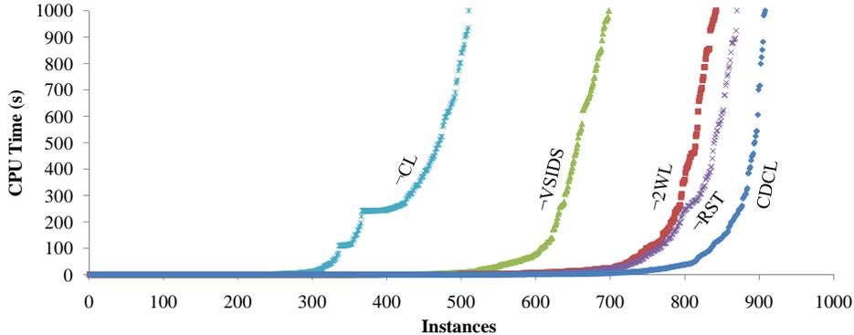
Fig. 3: The run time distribution of the four major CDCL features (data points for time-out runs are not shown to reduce clutter). These run times are averages over 10 runs per benchmark, and account for time-outs using *maximum likelihood estimation* (MLE) [32]. With a 90% confidence level, 71% of those averages are accurate to within 25%. Higher accuracy can always be obtained by increasing the number of runs.
